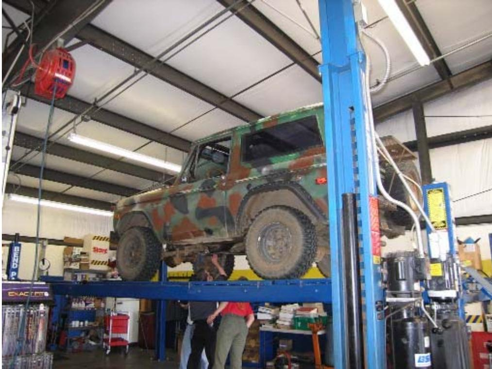
Ellen's YJ was next. We did a general inspection in the engine compartment and under the vehicle while it was on the rack. Torque the U-bolts to spec. (90 ft. Lbs). Ellen and Tom tuned her CB too. (Ed also adjusted the parking brake earlier.)
